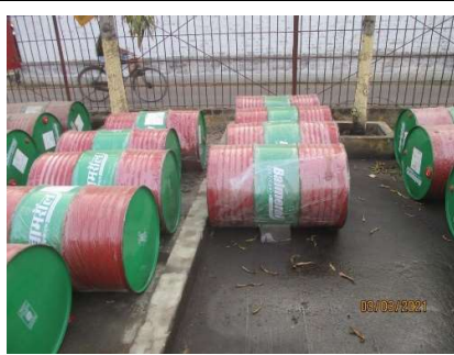
NC Photo # 11 Oil drums stored directly under the sunlight and rainwater, oil spills were observed on the ground and secondary containers not provided.
