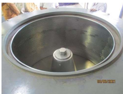
NC Photo # 6 Hydro machines do not have the lid and safety switch
