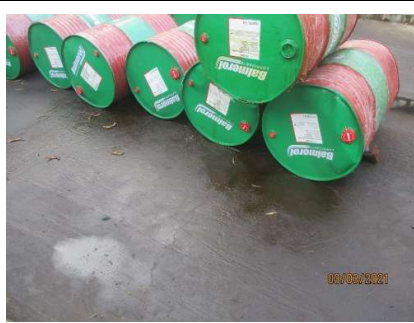
NC Photo # 11 Oil drums stored directly under the sunlight and rainwater, oil spills were observed on the ground and secondary containers not provided.
