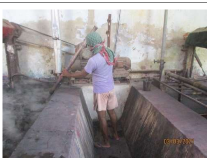
NC Photo # 6 Hydro machines do not have the lid and safety switch
