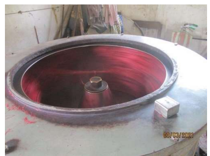
NC Photo # 6 Hydro machines do not have the lid and safety switch
