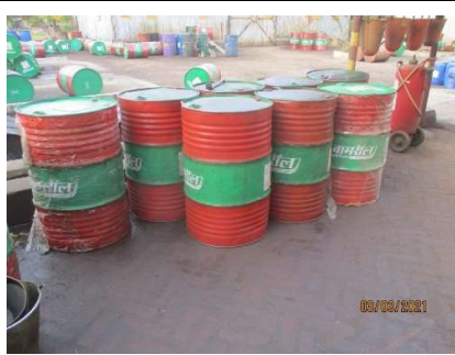
NC Photo # 11 Oil drums stored directly under the sunlight and rainwater, oil spills were observed on the ground and secondary containers not provided.
