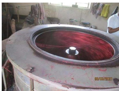
NC Photo # 6 Hydro machines do not have the lid and safety switch
