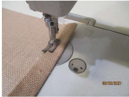
NC Photo # 8 Scissors and trimmers not secured, and needle guard not provided
