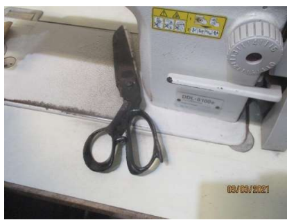
NC Photo # 8 Scissors and trimmers not secured, and needle guard not provided
