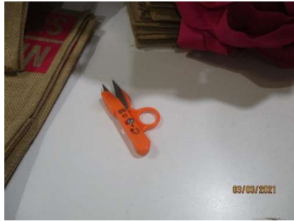
NC Photo # 8 Scissors and trimmers not secured, and needle guard not provided
